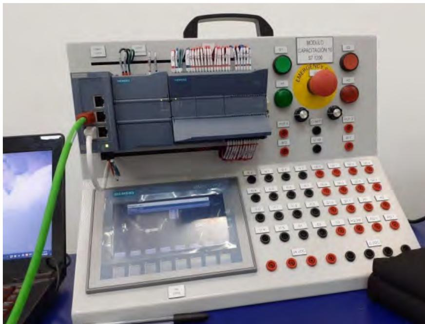
Figura 6.2: PLC Siemens S7-1200.
